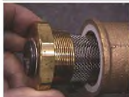
Remove the hose connection and drain the oil from here for 30 minutes
